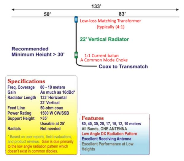
At this off-center feedpoint, a balun, usually 4:1 or 6:1, connects the coaxial feedline to the antenna, transforming the antenna's higher impedance of 200-300 ohms to match the 50-ohm feedline for efficient power transfer.
