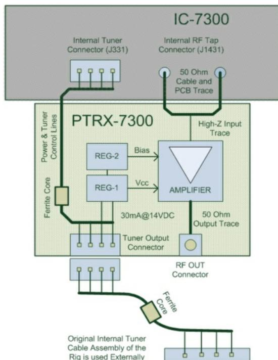
The PTRX-7300 board is professionally manufactured and equipped with high-quality components. A milled aluminium angle is used instead of the tuner socket of the IC-7300, which is routed to the outside with the supplied cables.
