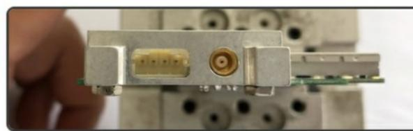
The current consumption is only 30 mA, leaving enough power for the external tuner. The installation only takes a few minutes, and a dismantling without residues is possible at any time without problems.
