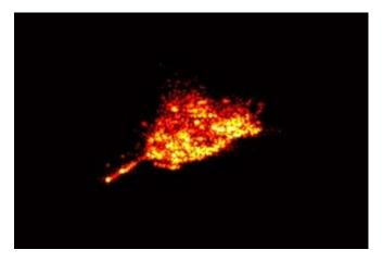
Radar image of the German ROSAT satellite a day before it re-entered earth's atmosphere uncontrolled. Taken by Tracking and Imaging Radar (TIRA) of the Frauenhofer Institute.
