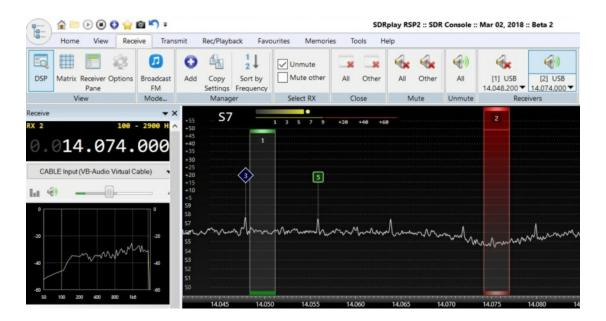
Then set the Audio Source of your digital modes decoder software to CABLE Output.
