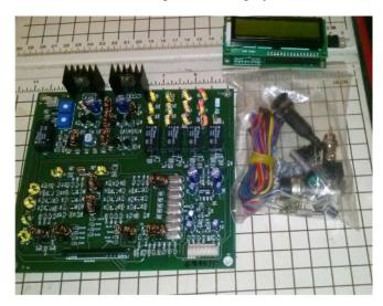
The  $\mu$ BITX uses upconversion to the first IF of 45 MHz which eliminates the need for a large number of band pass filters. The roofing filter at 45 MHz is 15 KHz wide. The signal is then down-converted to 12 MHz where a low ripple SSB filter with 8 crystals is used.
