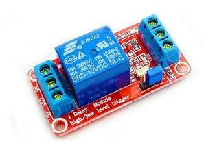
Upon wiring up the relay module to the 3.5mm 'SEND' output and a 12V supply I found the relay would not switch. I measured the output from the IC-705 and it did not change when I pressed the PTT. I then substituted the relay module with a simple 1K pull-up for the O/C output, still no change. I was then back digging into the ICOM user forum for advice, but no further comments were forthcoming.
