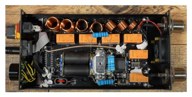
Looking inside the amplifier there is a 4-band Low Pass Filter fitted, there are two series inductors per band so a 4<sup>th</sup> order LC low-pass filter.
