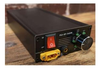
Its rather a simple device with manual band change and no RF switching. The label next to the 3.5mm socket on the front shows one pin is used for data but no further details were supplied nor is available from my internet searches. I bought the amp primarily to give my 10W signal an extra boost when I'm out in the car activating bunkers. As there is no RF switch, I had to make up a PTT interface from the 705.
